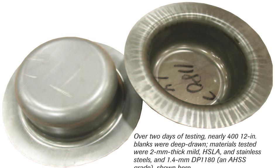
*Over two days of testing, nearly 400 12-in. blanks were deep-drawn; materials tested were 2-mm-thick mild, HSLA, and stainless steels, and 1.4-mm DP1180 (an AHSS grade), shown here.*
