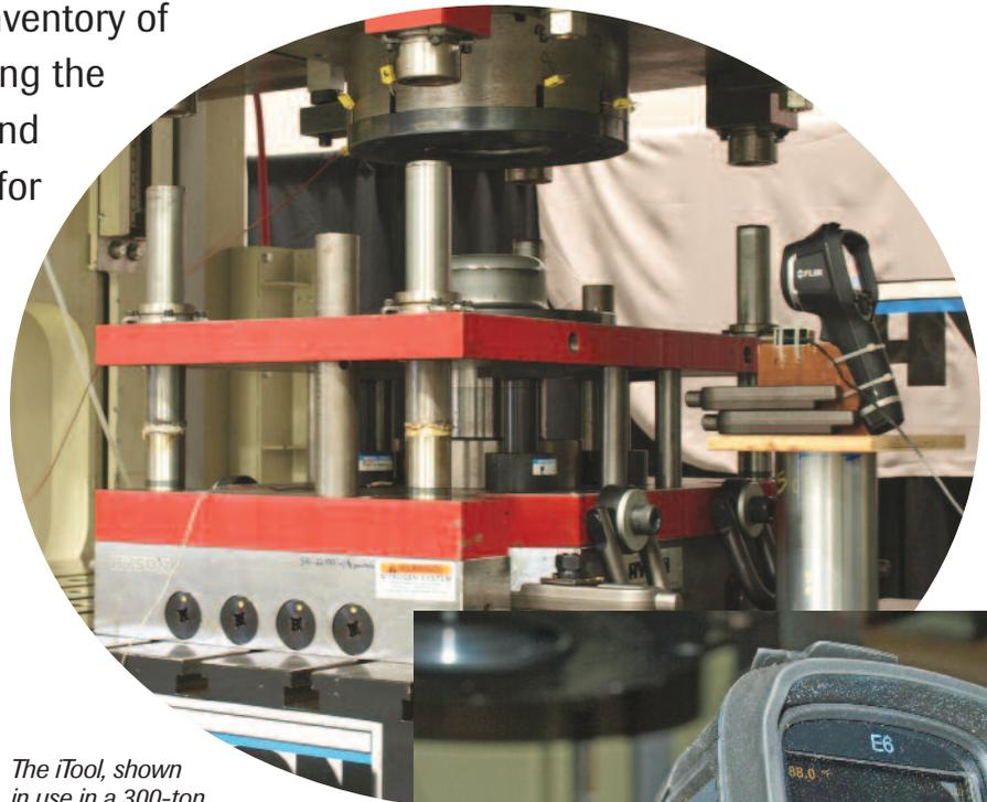
*The iTool, shown in use in a 300-ton Komatsu servo press at Hyson, is outfitted to measure and compare the frictional forces and deformation temperatures exhibited by one lubricant versus another. It features eight temperature sensors to monitor die temperature during testing, a load cell in the die, and an FLIR thermal-imaging camera (inset) to capture part-temperature data during drawing.*
